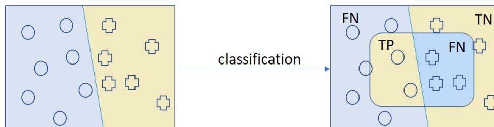
Figure 4.1: The visualization of confusion matrix for a binary classification task. There are two classes: circles and crosses. A small rectangle is a classifier that detects the samples inside it as circles and the samples outside it as crosses. The regions with yellow background depict correctly classified samples, the regions with blue background - mistakes of the classifier.
