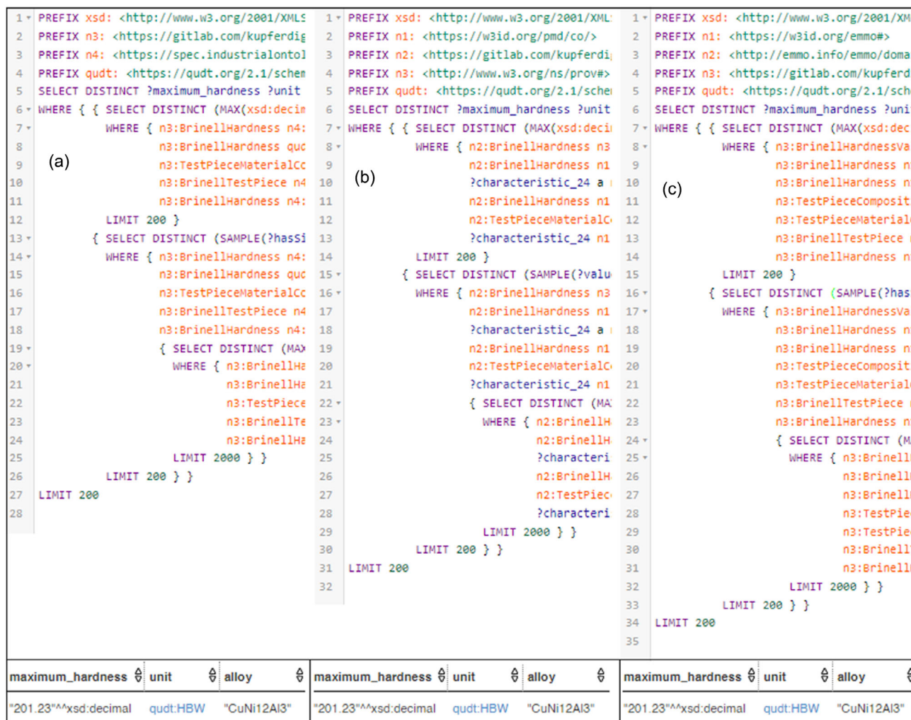
Figure 5. Apache Jena Fuseki-based SPARQL query for the alloy with maximum Brinell hardness (answer: CuNi12Al3 alloy with average Brinell hardness of 201.23 HBW) in different graphs: a- BTO 5.0.3 (BFO + IOF core+MSEO), b-BTO 4.0.3 (PROVO + PMDco), c-BTO 3.0.3 (EMMO + CHAMEO + MT).
